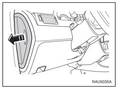
The instrument panel fuse block is located on the end of the instrument panel on the driver's side of the vehicle. To access the fuses, open the fuse panel door by pulling the door out.
